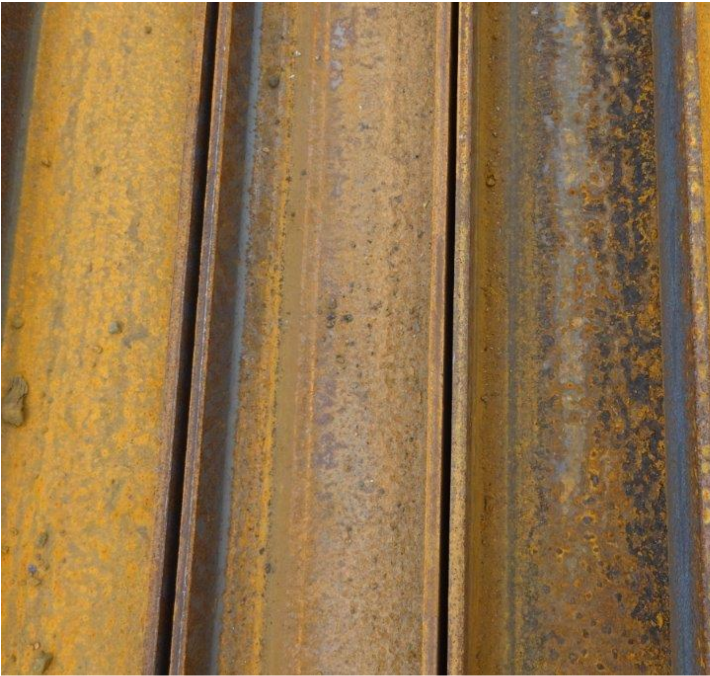
4 Mtrs 127 x 76 x 13 Universal Steel Beam RSJ
