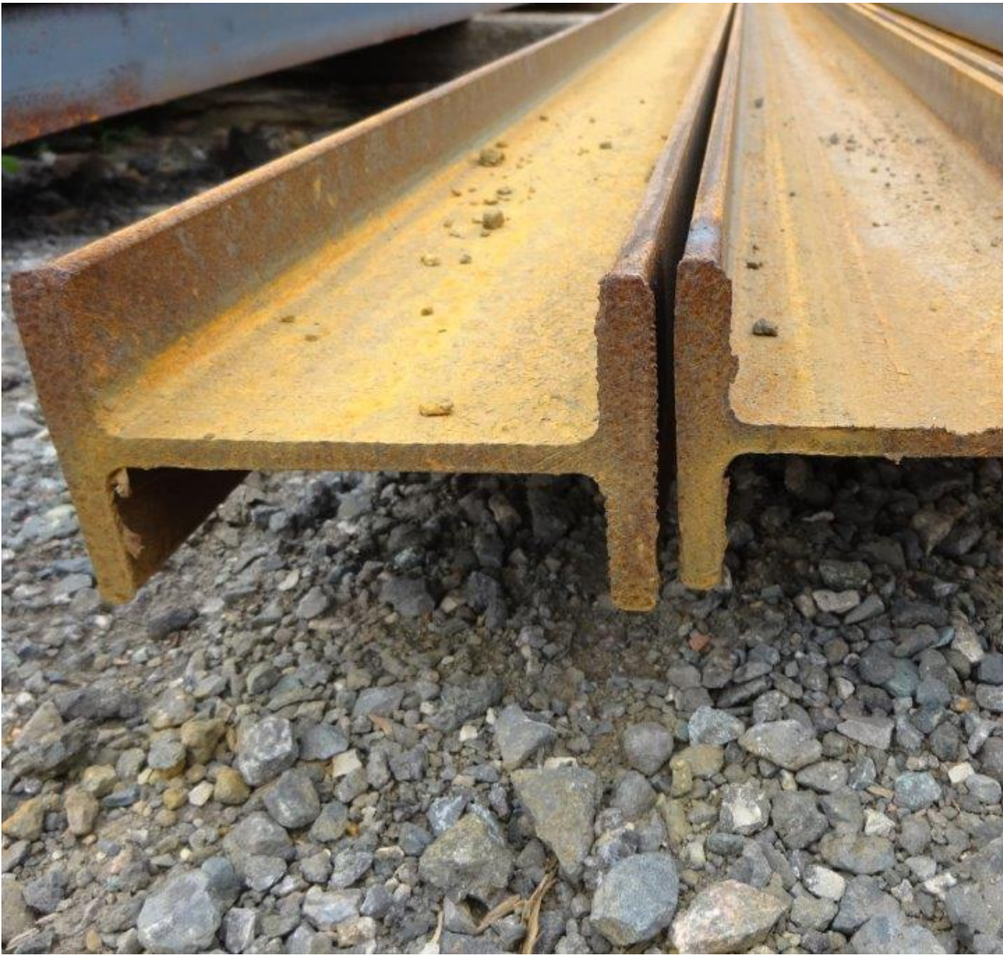
4 Mtrs 127 x 76 x 13 Universal Steel Beam RSJ
