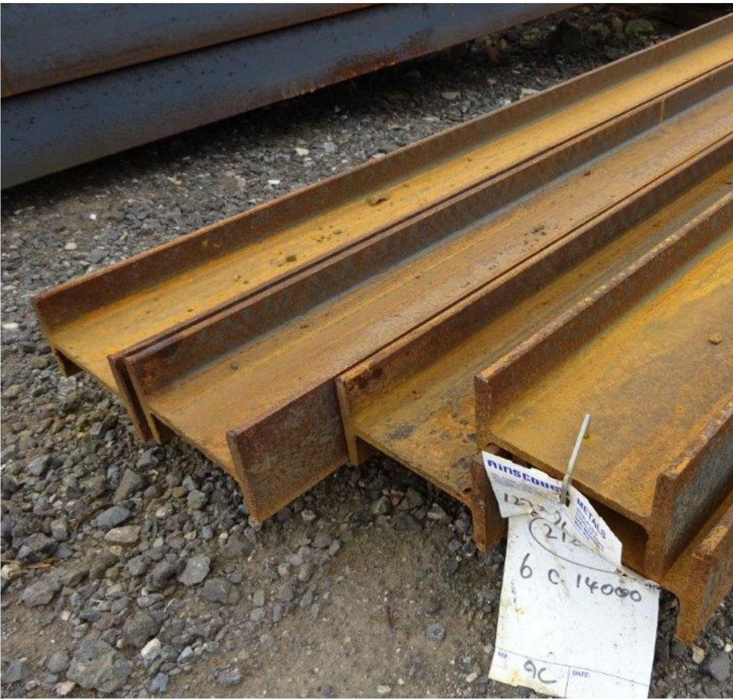
4 Mtrs 127 x 76 x 13 Universal Steel Beam RSJ
