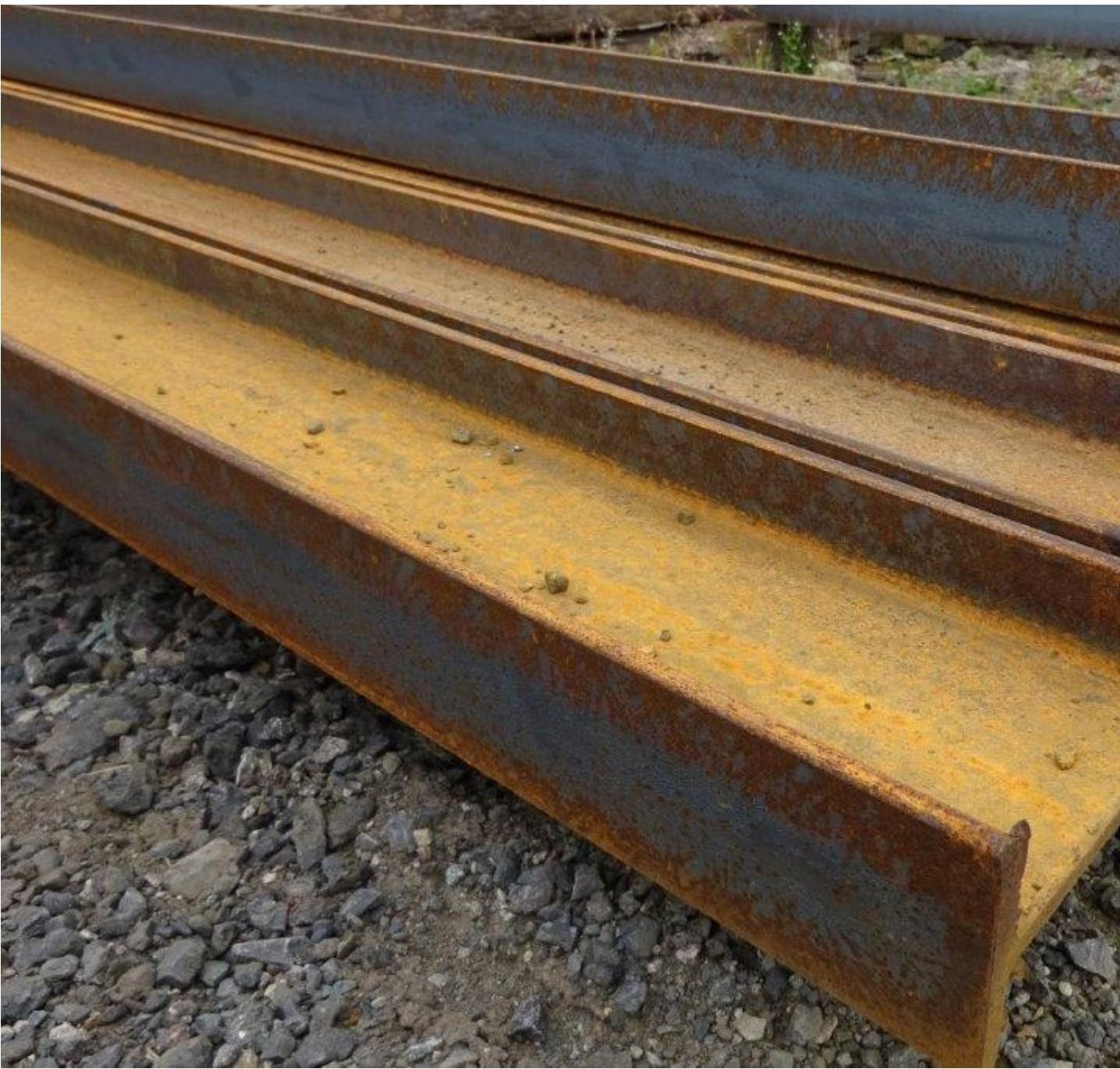
4 Mtrs 127 x 76 x 13 Universal Steel Beam RSJ
