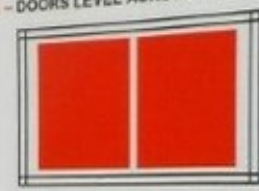
FIGURE 2 - DOORS NOT LEVEL
